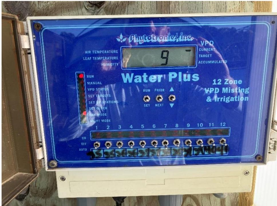
**Figure 14.** Phytotronics 12-zone vapor pressure deficit (VPD) controller.
