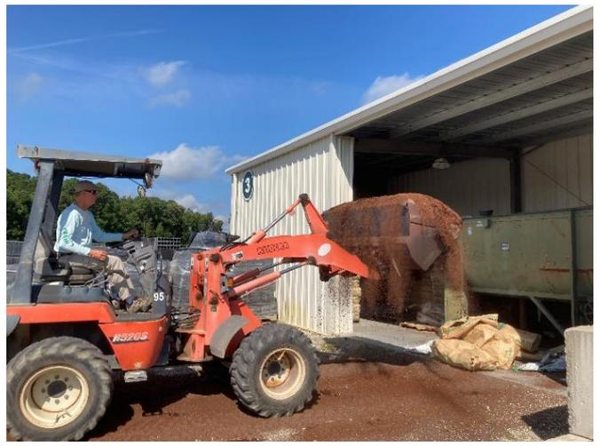
**Figure 9.** (left) Loading coarse perlite into 3.8 m<sup>3</sup> (5 yd<sup>3</sup>) paddle mixer, and (right) loading bulk aged loblolly pine bark into the paddle mixer.
