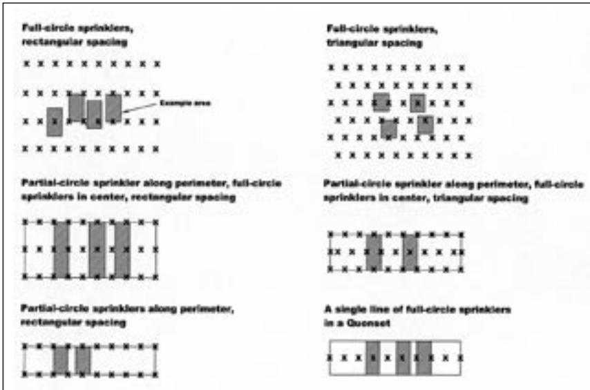
Figure 1. Areas containing a repeating water-distribution pattern.
