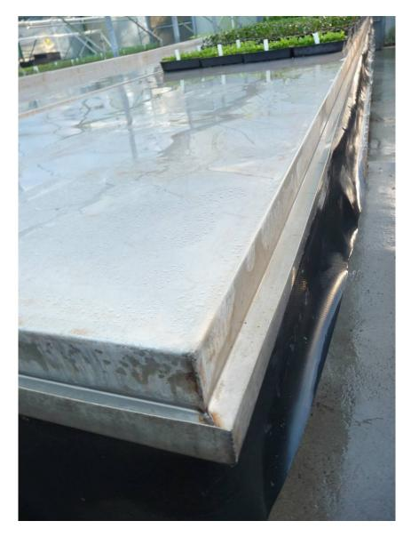
Fig. 8. Stainless-steel benches with side gutters, and plastic side curtains.
