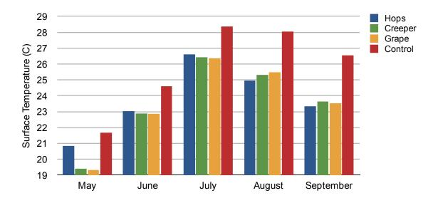
Fig. 4. Change in surface temperature over May to September 2013 behind the vegetated façades and the non-vegetated control walls.
