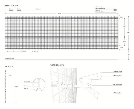
Fig. 1. A drawing of the greenscreen<sup>®</sup> 3D welded wire panel system.
