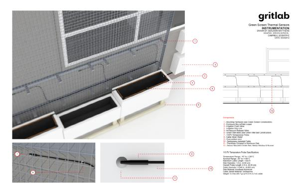
Fig. 3. Annotated drawing of the planter module.
