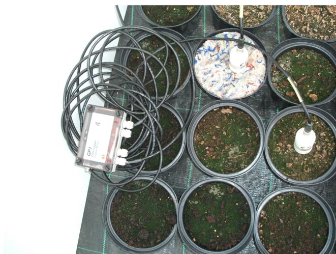
Fig. 4. Delta T moisture and temperature measurement equipment in place. Probes inserted in pot with pot cover and pot without pot cover.
