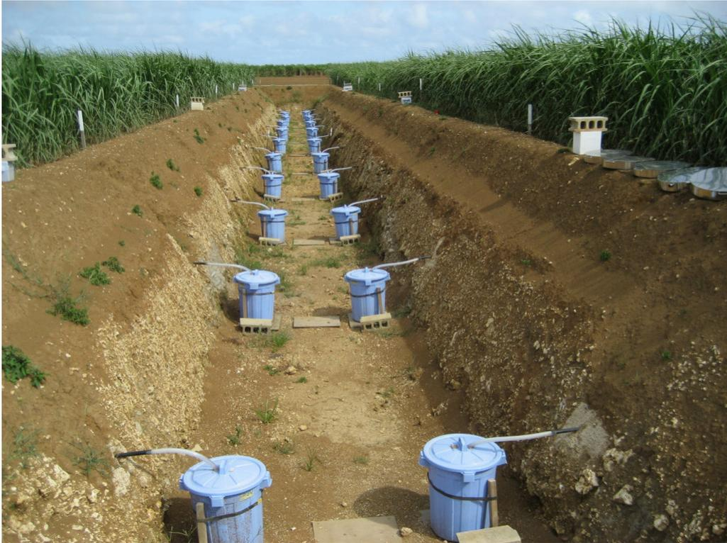
Fig. 2. Polyethylene tanks along the sugarcane field to collect soil penetration water.
