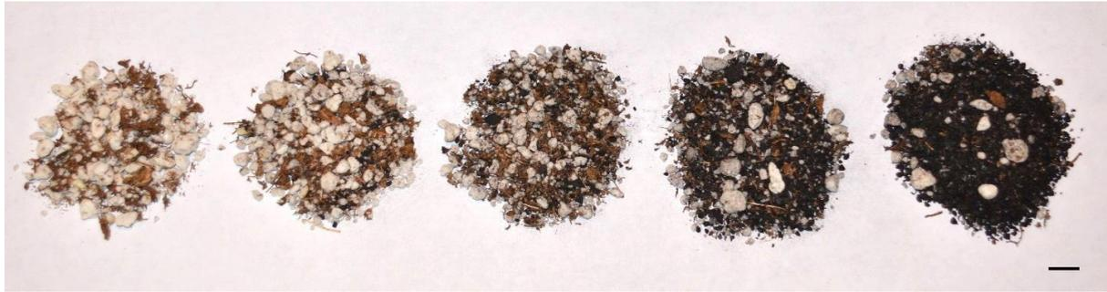
**Figure 2.** Sphagnum peat and coarse perlite (1:2, v/v) substrate amended with coconut-shell biochar at 0, 10, 20, 40, and 80% (left to right, v/v, bar = 1 cm).
