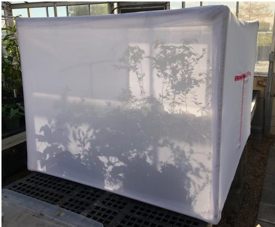
Figure 2. Plant chambers [1.3 m x 1.3 m x 1.2 m (4.2 ft x 4.2 ft x 3.8 ft)] containing fourteen plant species and cultivars.
