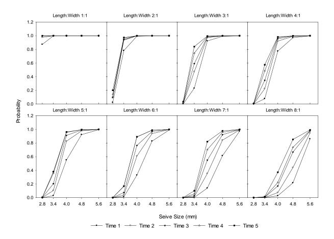
Fig. 2. Predicted cumulative distribution of 3 mm particles by length:width ratio and time.
