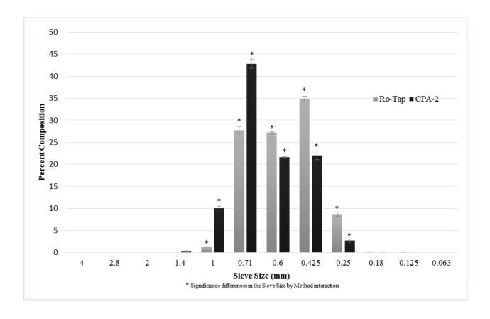
Fig. 4. Differential distribution of medium sand measured by Ro-Tap and CPA-2.
