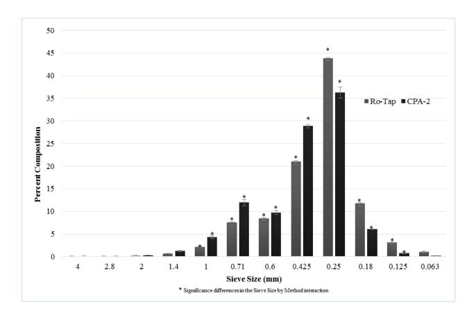
Fig. 5. Differential distribution of fine sand measured by Ro-Tap and CPA-2.
