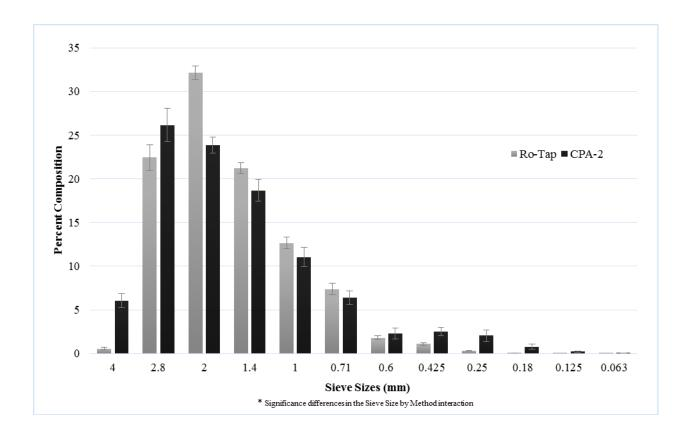
Fig. 3. Differential distribution of coarse sand measured by Ro-Tap and CPA-2.
