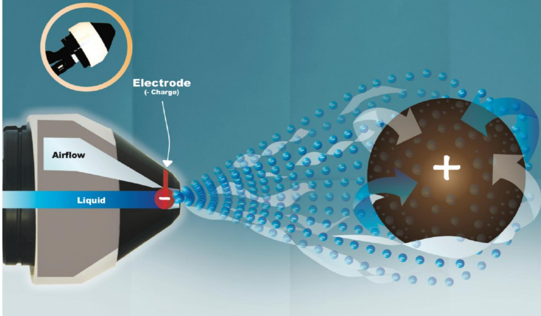
**STEP 1:** Separate liquid and air lines meet at the Maxcharge™ nozzle tip. The low pressure, high volume air flow quickly atomizes the liquid into uniform droplets. The small droplets then pass through an electromagnetic field. It is here that each droplet picks up a strong negative charge.
