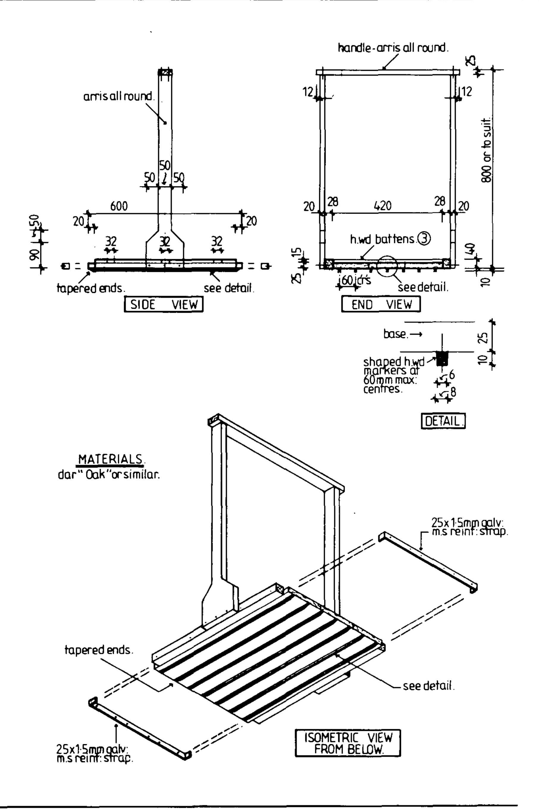
Figure 1. Diagram of drill-forming implement, the Northolme Nurseries Pty. Ltd. seed furrow presser.
