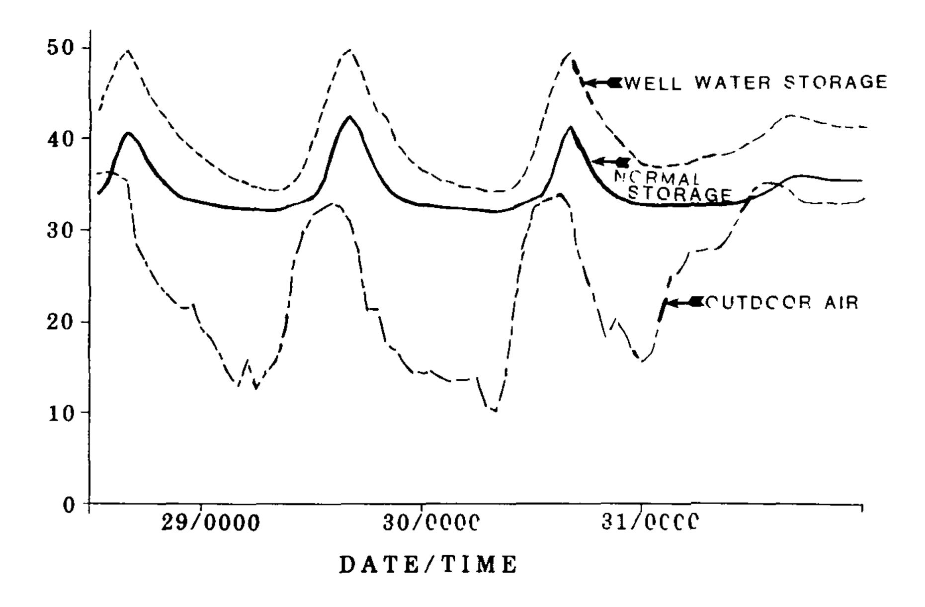
**Figure 3.** Medium temperatures under winter storage conditions in  $3 \times 3 \times 3$ . 3.5 in. cells.
