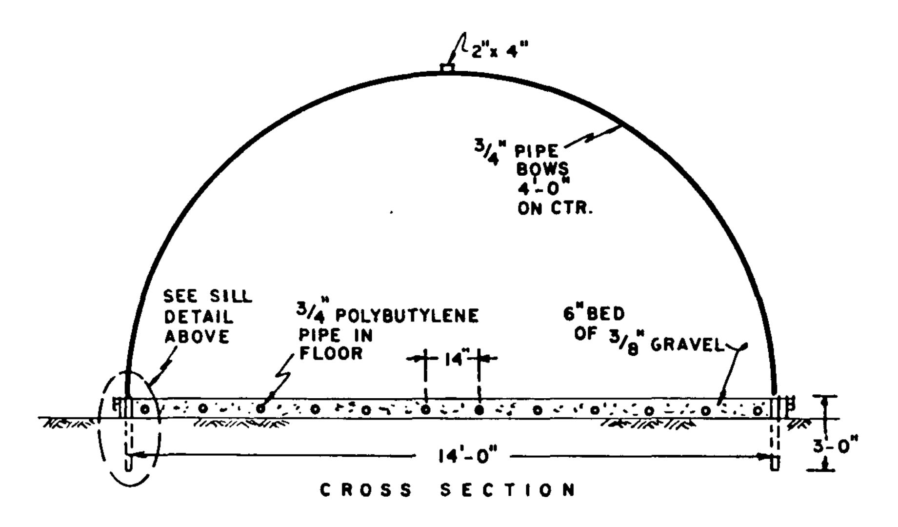
**Figure 1.** New Jersey Plan 153: Construction details of a floor heated nursery storage house.
