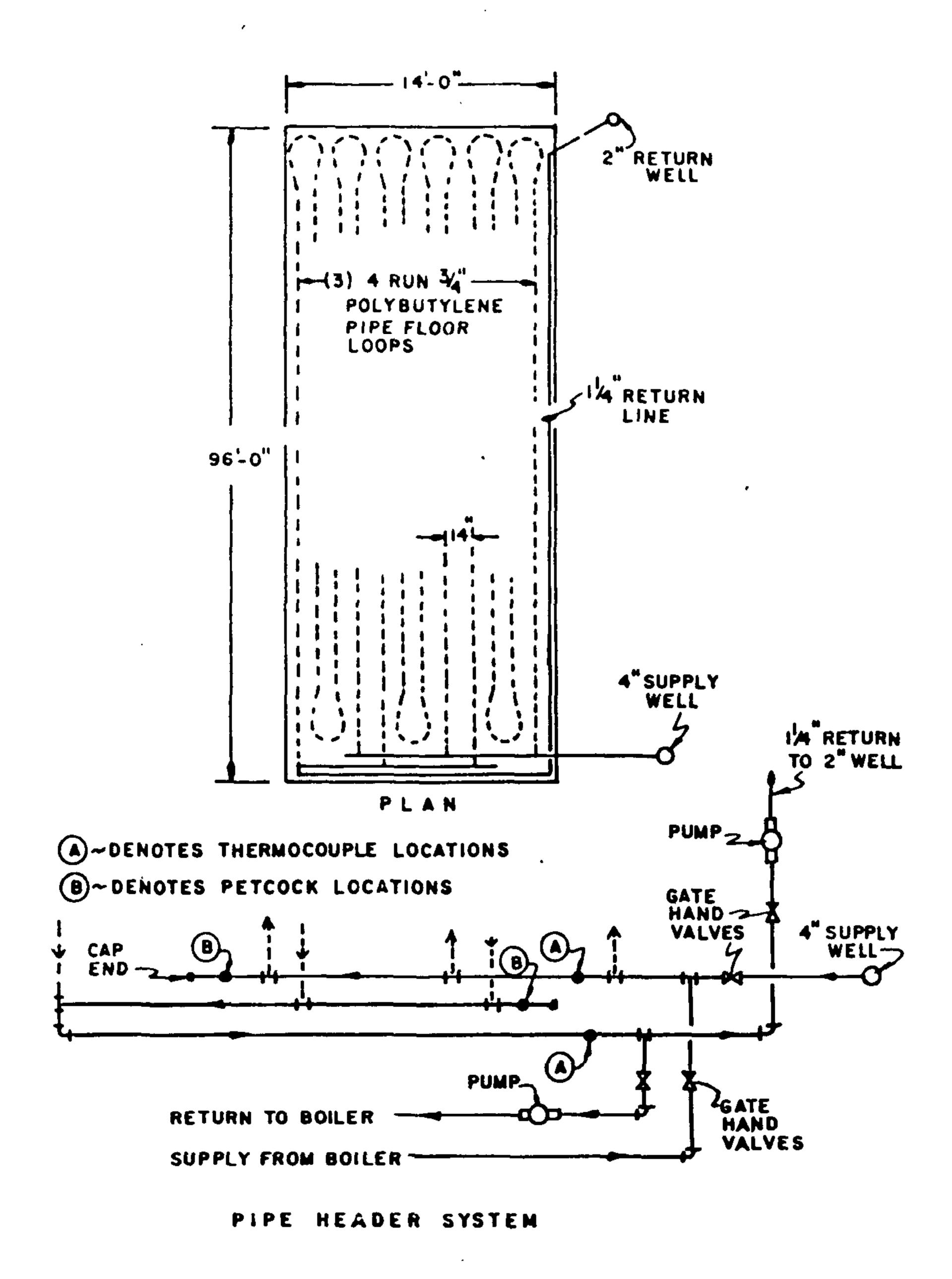
Figure 2. Engineering details for a heated floor incorporating a double-header return system.
