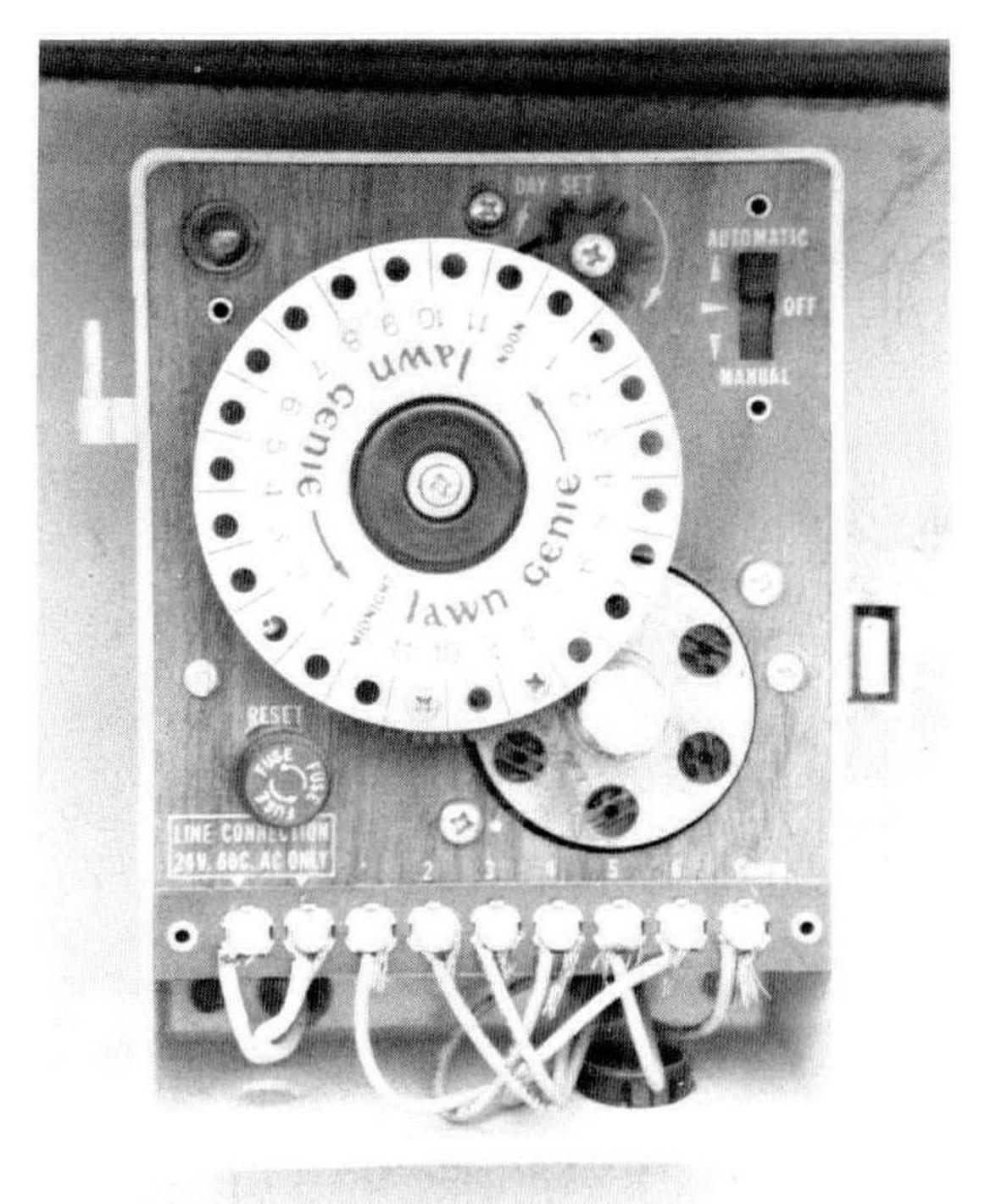
**Figure 1.** Richdel, Lawn Genie, 6-station lawn sprinkler controller converted into an inexpensive and flexible mist controller.
