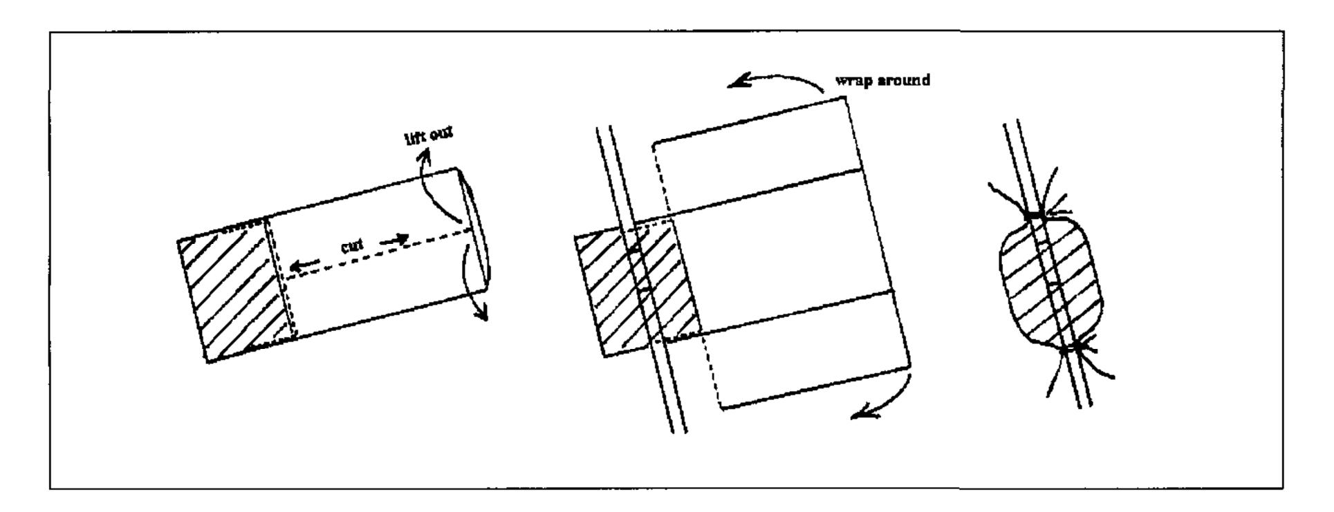
3) Pre-filled plastic bags tied off with 30 to 60 cm twine—plastic bags  $20 \times 10$  cm are pre-filled and the open end is tied off with 60 cm of strong twine. The plastic bag is cut from twine knot, along one side and down to the bottom. The rooting medium is pushed up around branch, plastic is pulled up either side of branch, over and around rooting medium. The plastic is then tied up using attached twine. Approximately 50/h can be completed.
