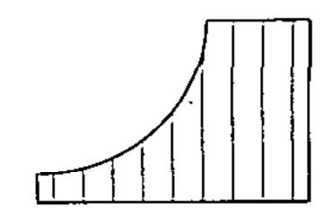
The vertical lines represent the dry bulb temperature (air temperature measured with a dry thermometer).
