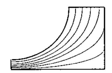
The curved lines represent the relative humidity of the air (amount of water vapour in air expressed as a percentage of amount of water vapour in 100% saturated air)
