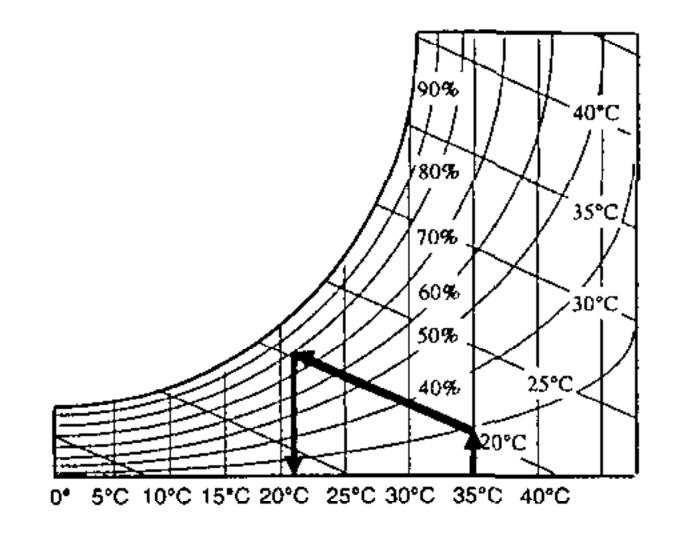
From the same chart, it is also possible to determine how much water would be required to cause that drop in temperature so that a fogging system could be designed to perform the task.
