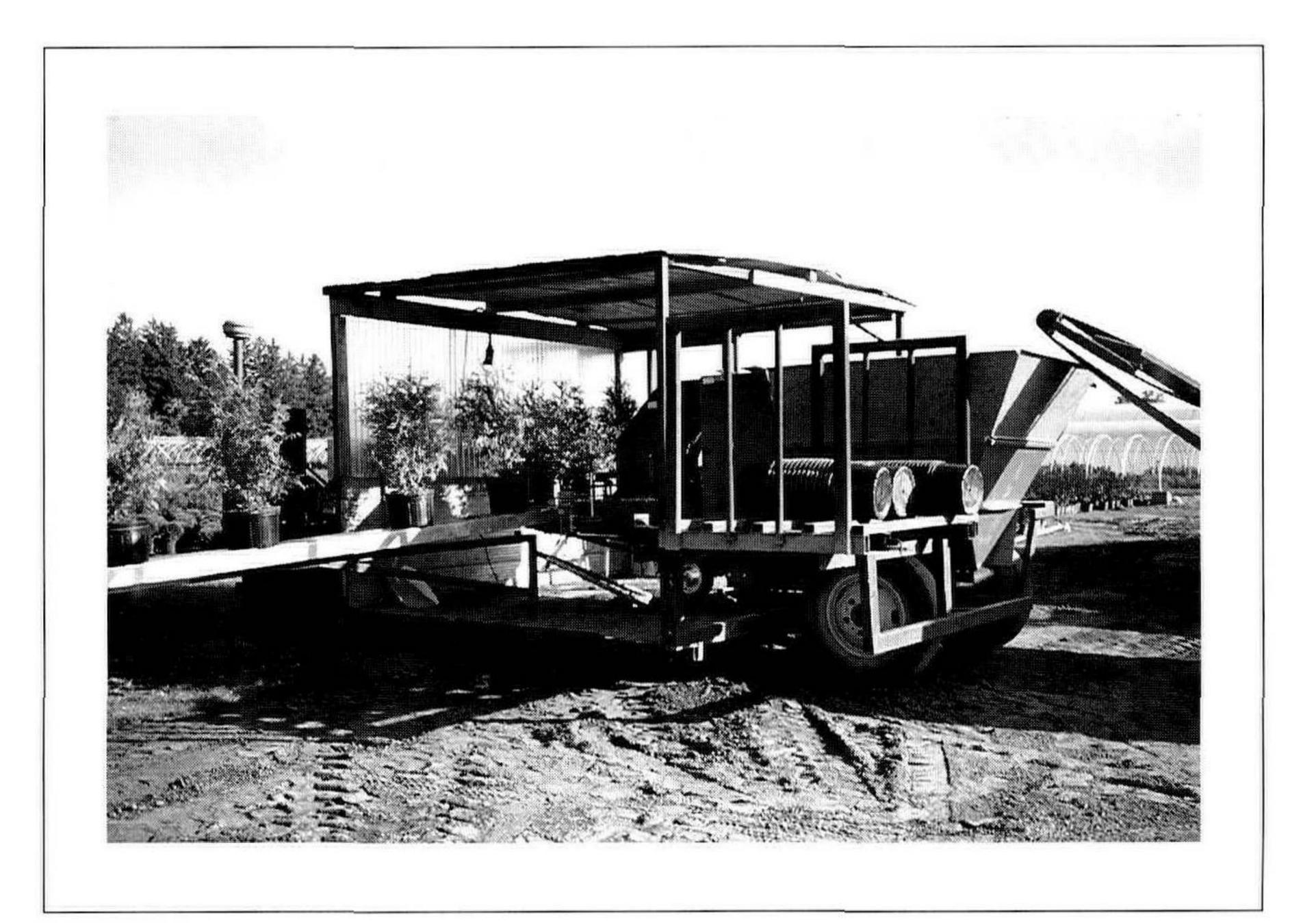
Figure 1. Portable potting machine.
