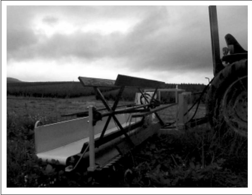
**Figure 1.** Tractor-mounted device including a conveyor for harvesting biomass.
