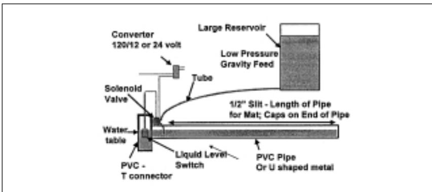
**Figure 3.** An electric control system to control the level of water in the trough.
