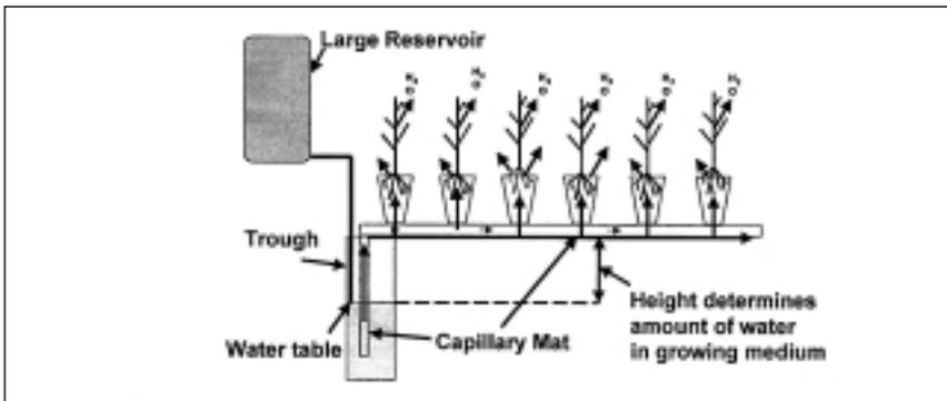
**Figure 1.** Controlled water table irrigation system.
