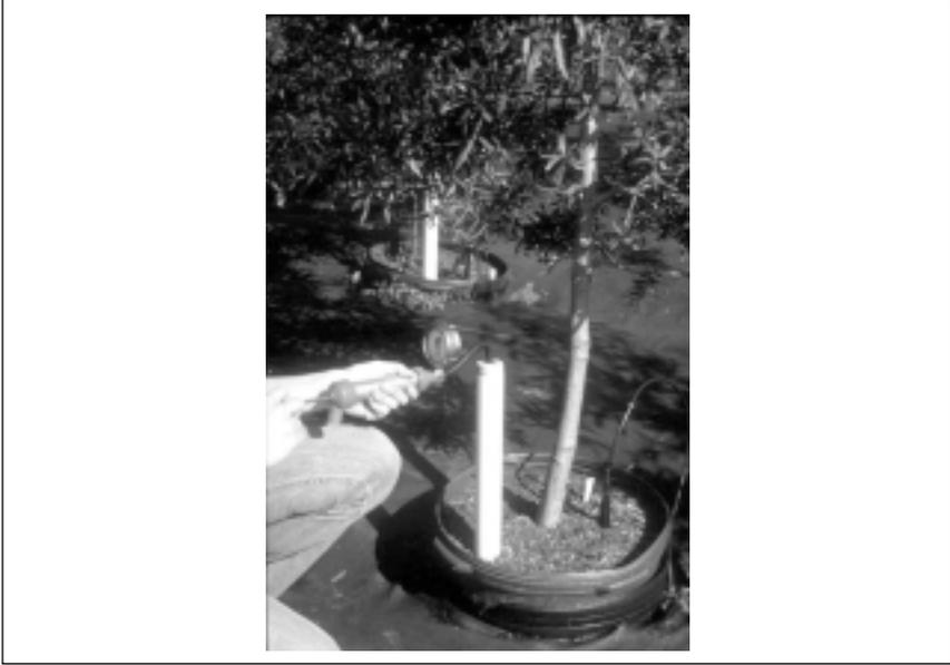
**Figure 2.** Vacuum being drawn on a suction cup lysimeter in a 57-liter (15-gal) in-ground container.
