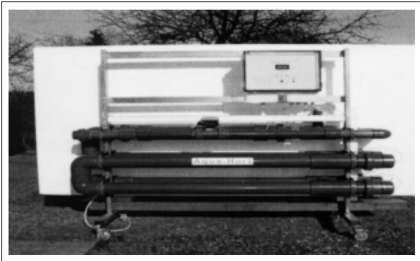
**Figure 1.** Aqua-Hort system. The electromagnetic pipe, flow meter, and conductivity sensor are located above the four electrode pipes.
