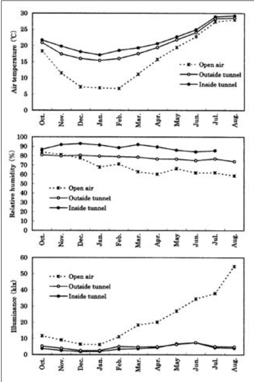
Figure 2. The change of air temperature, relative humidity and illuminance. The data is the monthly average.
