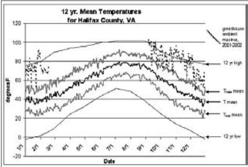
Figure 1. Ambient temperature data for Halifax County, Virginia, including 12-year mean, maximum, minimum, record high and low, and ambient tobacco greenhouse temperature (broken line).
