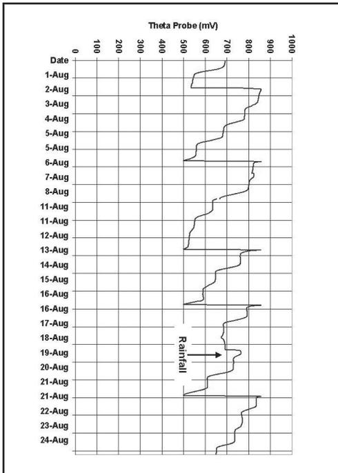
Figure 4. Theta probe output triggering irrigation.
