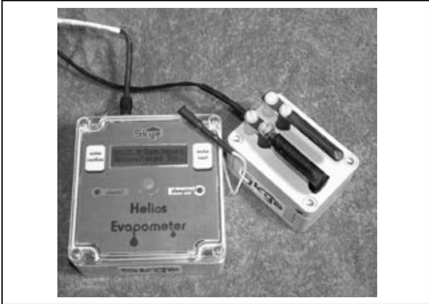
**Figure 1.** Skye Evapometer and Evaposensor.
