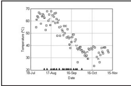
**Figure 4.** Temperatures during composting of green waste, sawdust and spent black brewer's grain (triangle symbols mark turning dates).
