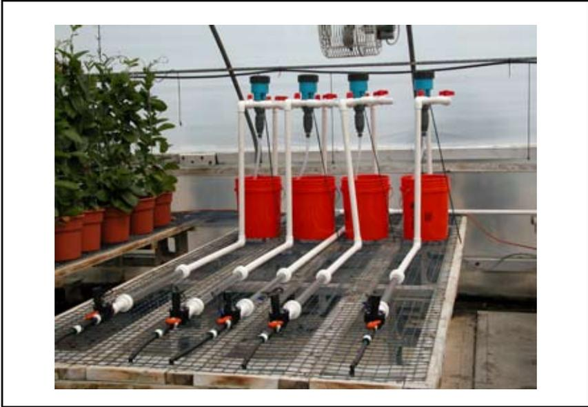
**Figure 8.** Experimental irrigation matrix for researching biofilm and algae in irrigation lines.
