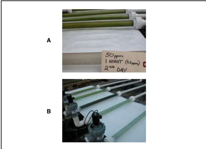
**Figure 10A & 10B.** Top image showing clear section of line following shock treatment with Selectroicide. Bottom image showing various treatments with untreated control line in center. Note algae contamination in center line.
