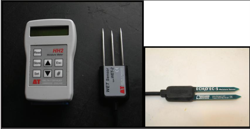
**Figure 2.** Moisture sensors, such as this hand-held sensor and meter (WET Sensor, Delta T Devices; left) and in-situ sensors (EC-5, Decagon Devices, right) effectively measure substrate moisture content and may be used to monitor or automate irrigation of rooted plants in containers as small as 10-cm pots. However, they are too large for use in propagation.
