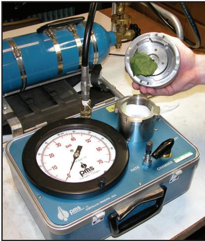
Figure 8. Pressure chamber to measure hydraulic conductivity.
