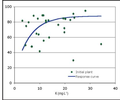
**Figure 6.** Plant coverage and potassium in saturated media extract test results of 30 established green roofs.
