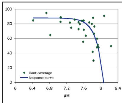
**Figure 2.** Saturated media extract sample pH and plant coverage for 30 green roofs.
