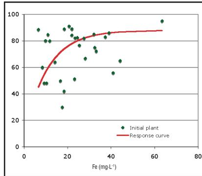
**Figure 9.** Plant coverage and iron in saturated media extract of 30 sampled green roofs.
