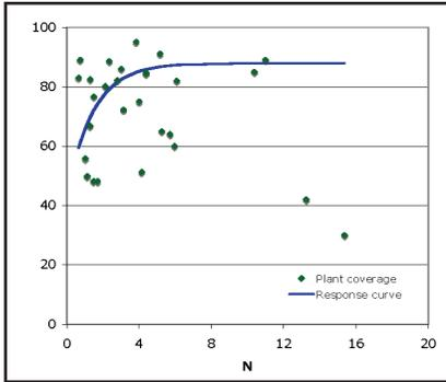
**Figure 3.** Nitrogen (nitrate + ammonium) in saturated media extract of 30 sampled green roofs and plant coverage.
