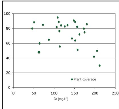
**Figure 7.** Plant coverage and calcium in saturated media extract of 30 sampled green roofs.
