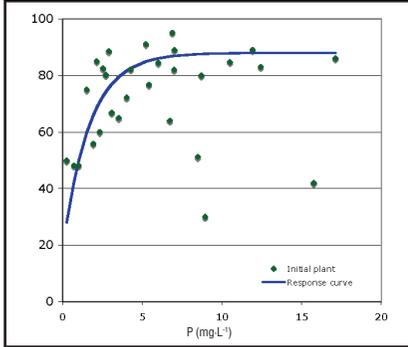
**Figure 5.** Plant coverage and phosphorus in saturated media extract tests of 30 existing green roofs.
