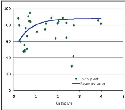
**Figure 8.** Plant coverage and copper in saturated media extract of 30 sampled green roofs.
