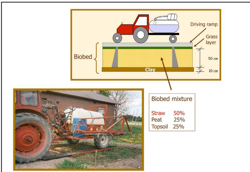
**Figure 1.** Biobed developed by University of Sweden (Castillo and Torstensson, 2008).
