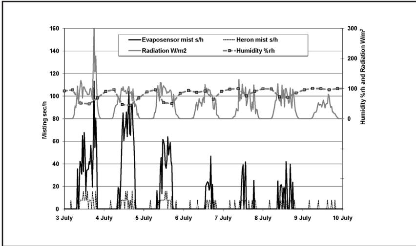
**Figure 3.** Lowaters Nursery. Half-hourly plots of misting and ambient environment July 2008, showing the sensitive response of Evaposensor control.
