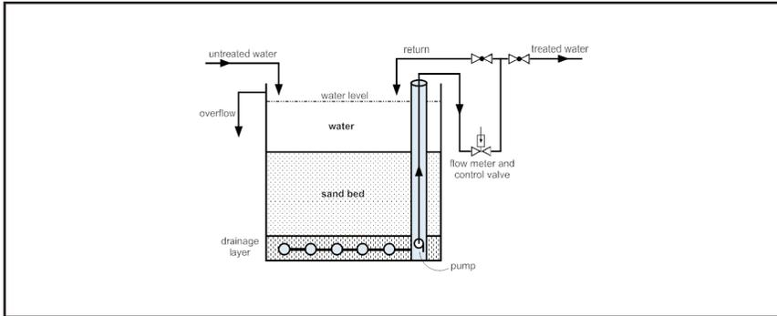
**Figure 1.** Slow sand filtration system showing sand bed, under drain layer, and pump. Flows are monitored and controlled to optimize treatment. When untreated water levels are low, treated water is returned to the filter to keep the sand bed submerged.
