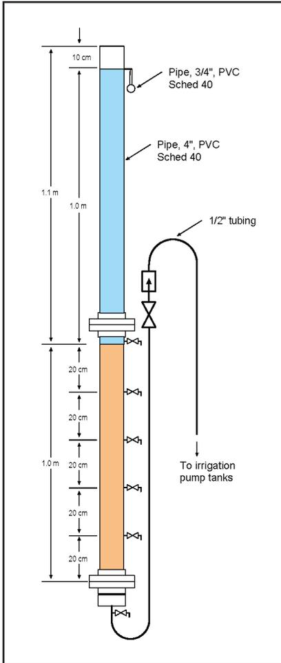
**Figure 2.** Sand filters for experimentation were constructed of 4-ft PVC pipe and included valves that enabled collecting samples above the sand bed, at 20-cm intervals down the sand bed, and below the bed.
