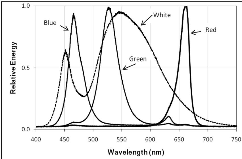
**Figure 3.** The spectral distributions of LEDs. Coloured LEDs (red, blue, and green) emit defined, relatively narrow, spectra of light energy. The LEDs perceived as white to the human eye are blue LEDs modified with phosphor to produce a wider spectrum peaking in the yellow wavelength band (550 nm). For direct comparison, the energy levels have been scaled to show the relative distribution of each light source.
