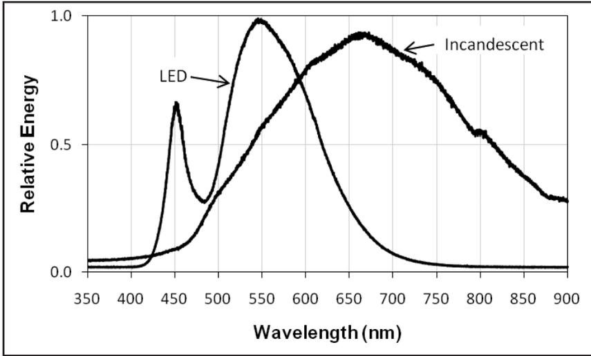
**Figure 4.** Spectral distributions for two white light sources. In contrast to the white LED, the incandescent lamp has a much wider spectrum, emitting a significant portion as non visible, infrared (>750 nm), radiation, which is experienced as heat. For direct comparison, the energy levels have been scaled to show the relative distribution of each light source.
