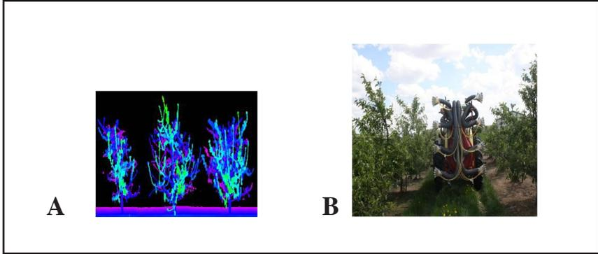
**Figure 2.** Laser-scanning sensor-controlled air assisted sprayer to provide variable-rate functions based on tree sectional canopy volume, density and occurrence
