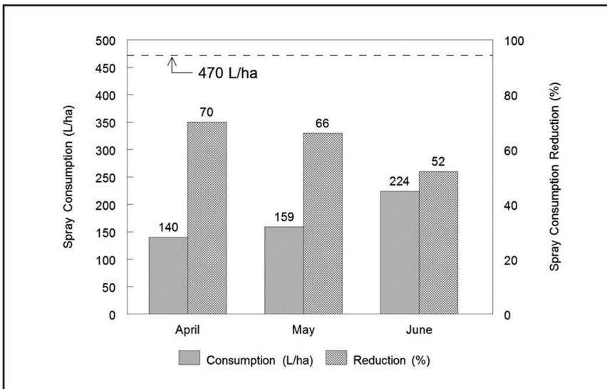
**Figure 3.** Spray consumption and percent reduction from intelligent sprayer, compared with the conventional 470 L·ha<sup>-1</sup> (50 gpa) spray application rate.
