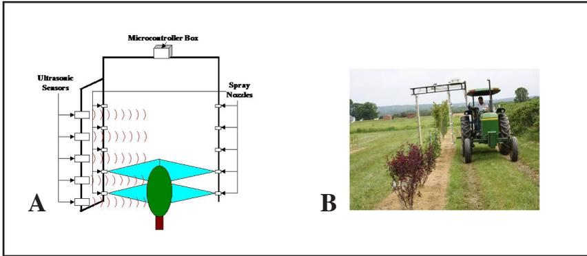
**Figure 1.** Ultrasonic sensor-controlled hydraulic vertical boom sprayer to provide variable-rate functions based on tree size, shape, and occurrence.
