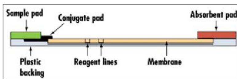
Fig. 2. Diagrammatic representation of the Pocket® Diagnostic™ test kit (Source: IVD Technology).
