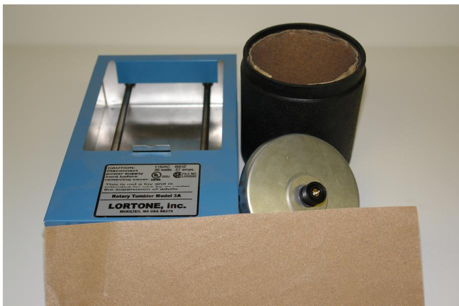
Fig. 8. Small batch seed scarifying equipment.
