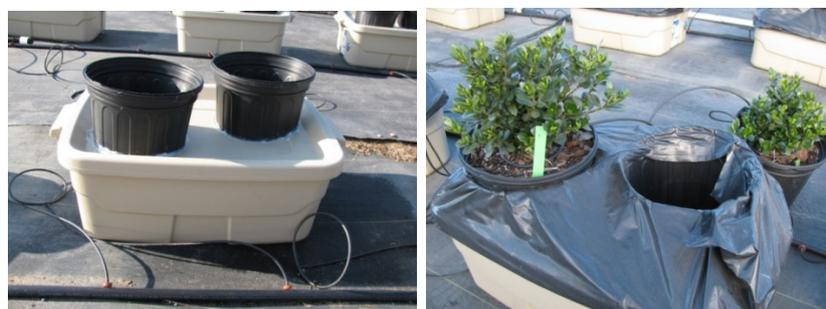
Fig. 1. The setup for leachate collection/rainfall exclusion.
