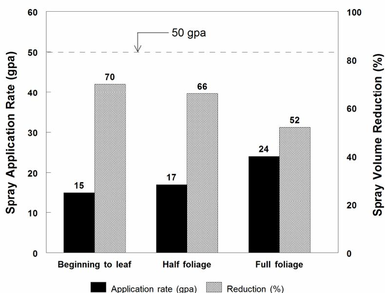
Fig. 1. Spray application rate and percent spray volume reduction from intelligent sprayer, compared with the conventional 50 gpa spray application rate at beginning to leaf, half foliage and full foliage stages.
