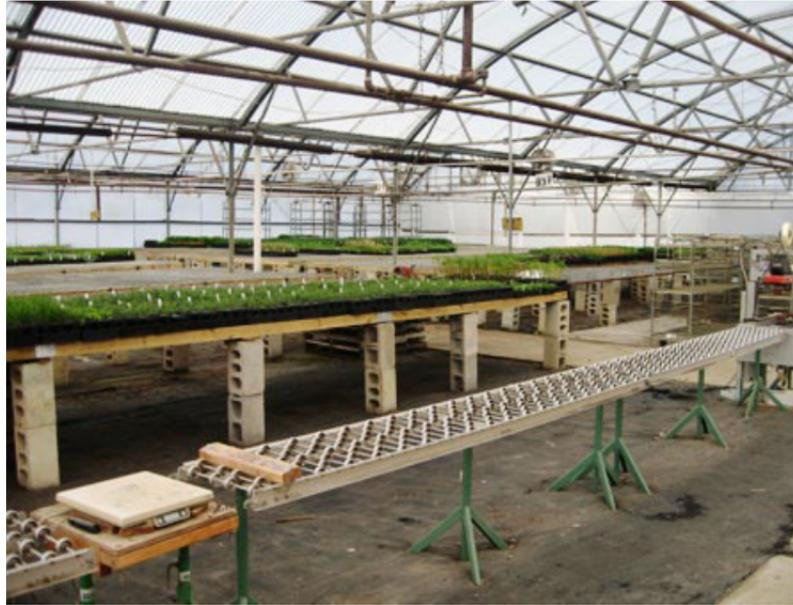
Fig. 4. Central location in the shipping greenhouse where a production line was employed to clean and organize materials and made ready for shipment.
