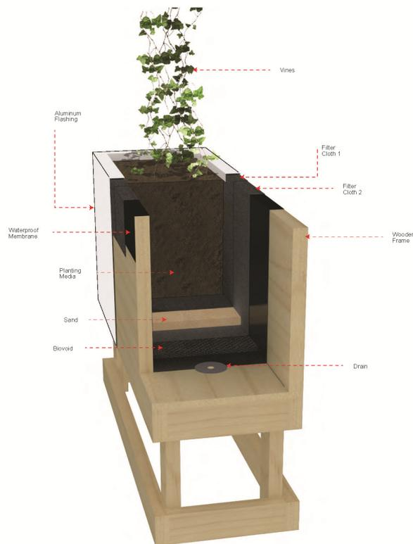
Fig. 2. Annotated drawing of the planter module.
