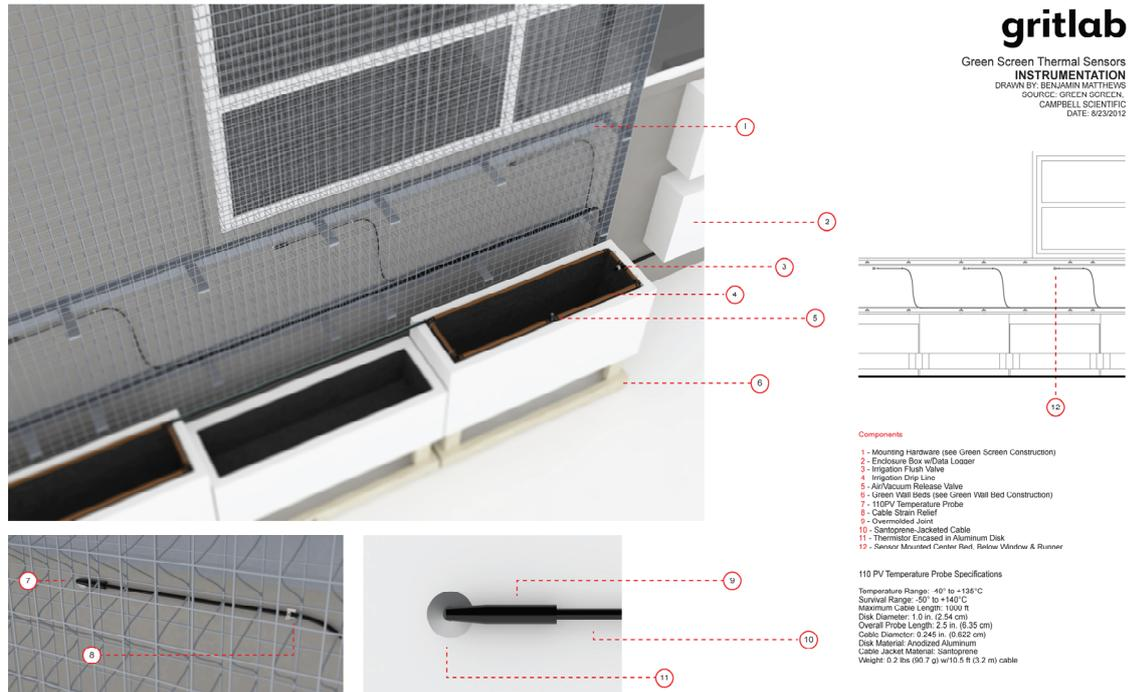
Fig. 3. Annotated drawing of the planter module.
