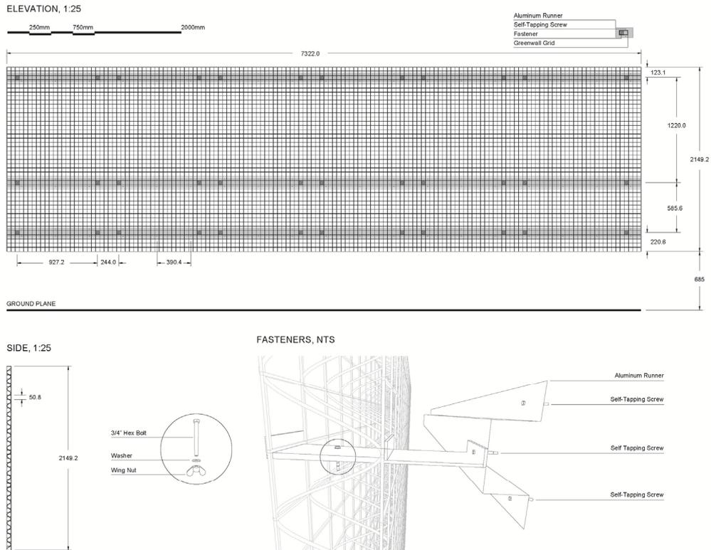
Fig. 1. A drawing of the greenscreen<sup>®</sup> 3D welded wire panel system.
