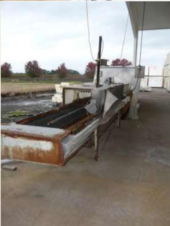
IFA run trays through high pressure jets to clean, then sterilise trays at 180°F (82°C) before packing and storing. Trays are then steam sterilised before use
