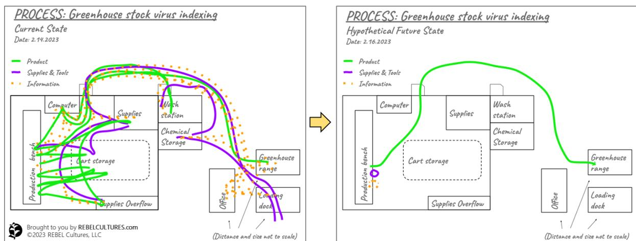
**Figure 2.** Diagrams of the current state of a process, including the flow of information, supplies and tools, and products in contrast with a hypothetical future state of the same process, focused exclusively on the highest value step(s).
