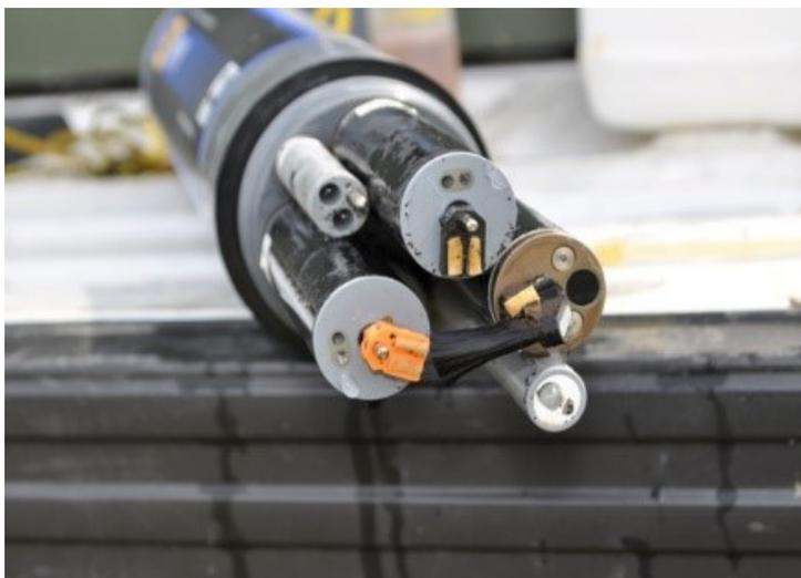
Figure 1. A multiprobe Sonde set to continuously monitor water quality.
